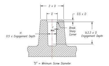
Hole sizes for the plastics listed in the table are derived by multiplying the minimum screw diameter by the factor listed in the table. The resulting hole size should be considered as a starting point which may need to be adjusted due to specific application conditions.
